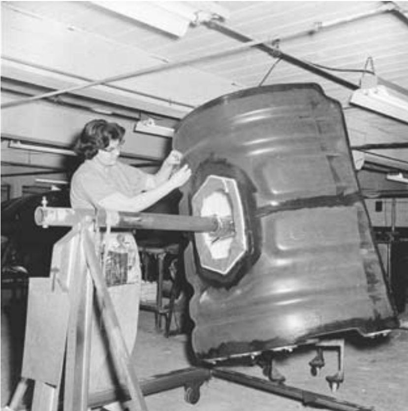
Magnolia's Firestone plant produced parts for military planes, submarines, armored vehicles and civilian vehicles during the 1960s. In this 1965 photo, Mary Frances Dodson works on an aircraft fuel cell.
